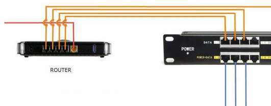
Injector connection to router/switch/nvr
