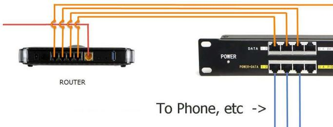
The POE side of the injector goes to the camera, phone or wifi access point. The LAN side goes to any Ethernet switch. Connect the 12 volt adapter to the 8 port injector. One LAN cable is needed for each POE port in use.
