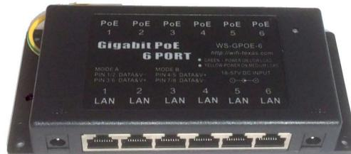
WS-GPOE-6 with Mode A or B power inputs
